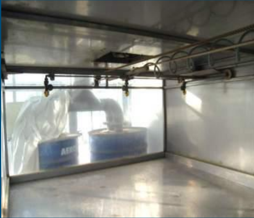
Spray cabinet with nozzles
